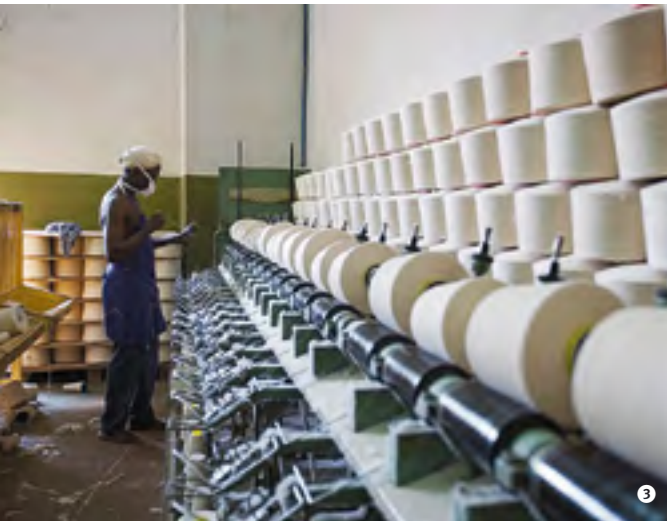
❶ The cotton undergoes initial sorting in the fields. ❷ The mills spin the bales of cotton into yarn many metres long. The grade and quality of the cotton are constantly checked during spinning. ❸ The cotton is wound onto large bobbins and is now ready for the next stage of processing, namely weaving.
